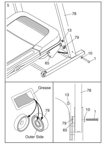
6. **See the left inset drawing.** Identify the outer side of the remaining Frame Spacer (79).
